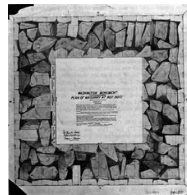
Cross section of rubble in shaft at 150 feet and typical of rubble below 150 feet
