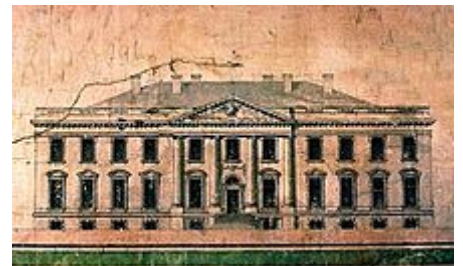
A 1793 elevation by James Hoban . His 3-story, 9-bay original submission was altered into this 2-story, 11-bay design.
